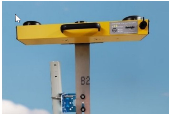
Example T-mount Installation on Flat Reference Surface
